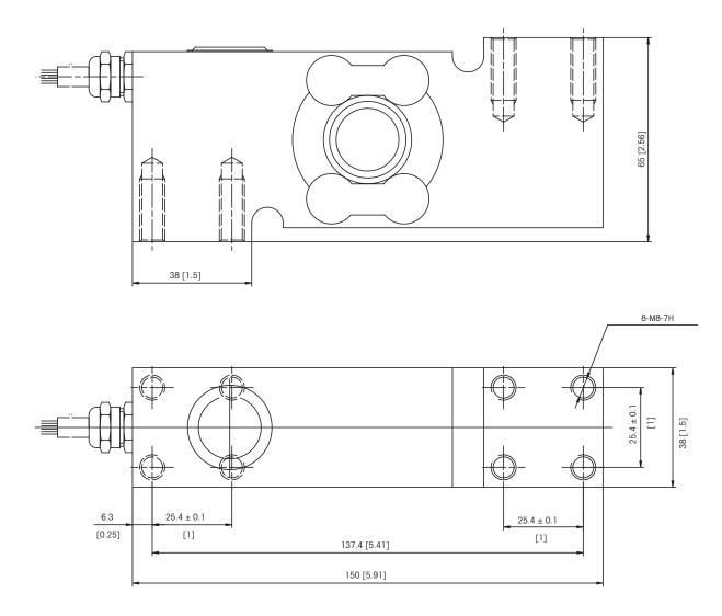
SSH 1000kg Load Cell Dimensional Drawings mm [inch]
