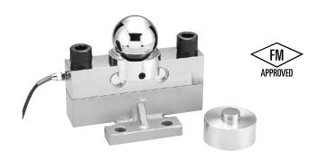
MDB is constructed of alloy steel and is fully potted and sealed with special chemical compounds to IP67 providing excellent protection against water and moisture attack. MDB Hermetically-Sealed is constructed to IP68 providing excellent protection against corrosive and wash-down environments.
